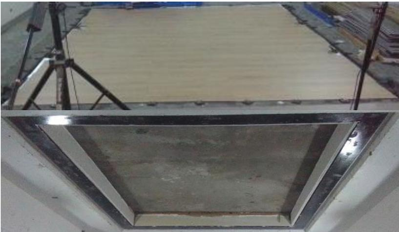
*Photo 1: View of Source Chamber, Urban Surfaces SoundTec SPC finish flooring installation observed*
